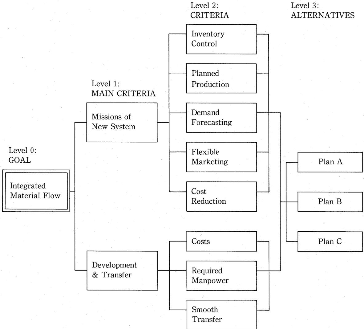
construct an integrated system which covers information about the flows of raw materials, products in process and inventory at factory stock room, distribution centers, and retail stores. At this stage, the hierarchy shown in Figure 3 was drawn. This chart consists of five levels, and was too complicated for the initial stage of planning.
