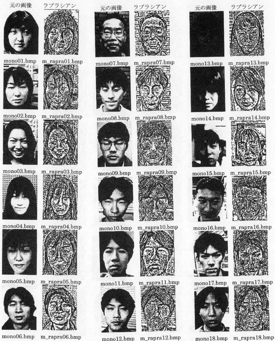
Fig.A2.1 18 original face-images \varphi_n(x, y) and the corresponding images \eta_n(x, y) = \partial^2 \varphi(x, y) / \partial x^2 + \partial^2 \varphi(x, y) / \partial y^2 ( n=1 \sim 18 ) (\varphi_{**} = \text{mono} ** .\text{bmp}, \eta_{**} = \text{m\_rapra} ** .\text{bmp}, x = x_1, y = x^2) .
